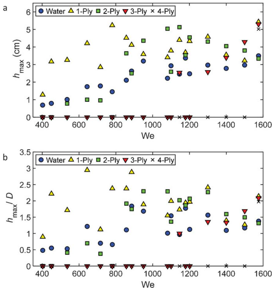
**Figure 3. Splash heights across Weber number ( $We$ ).** (a) Worthington jet height  $h_{max}$  vs.  $We$ , with  $h_{max}/D$  vs.  $We$  shown in (b). Number preceding "Ply" denotes the layers of fabric. [Please click here to view a larger version of this figure.](#)
