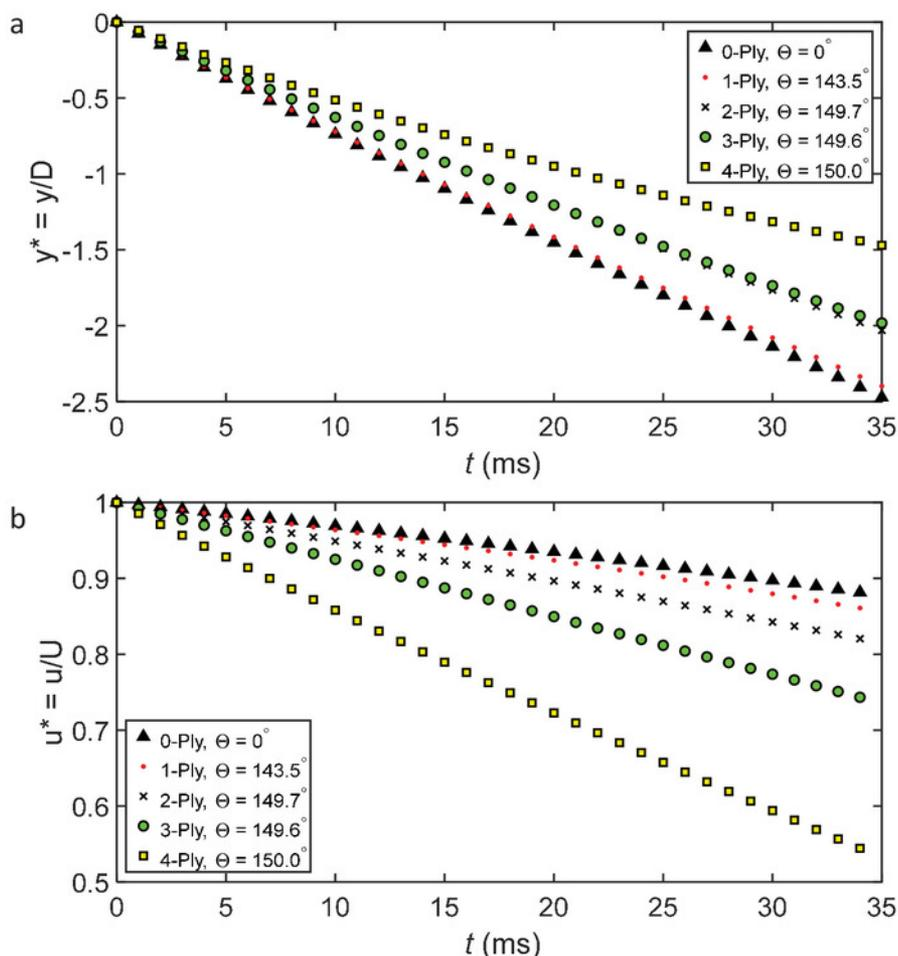
**Figure 5. Representative kinematics of sphere during underwater descent.** Temporal tracks of (a) vertical position  $y$  and (b) velocity  $u$  for impacting spheres with 0- to 4- layers of fabric atop the water. Trajectories are non-dimensionalized in terms of the sphere diameter,  $D$  and impact velocity  $U$  respectively. [Please click here to view a larger version of this figure.](#)
