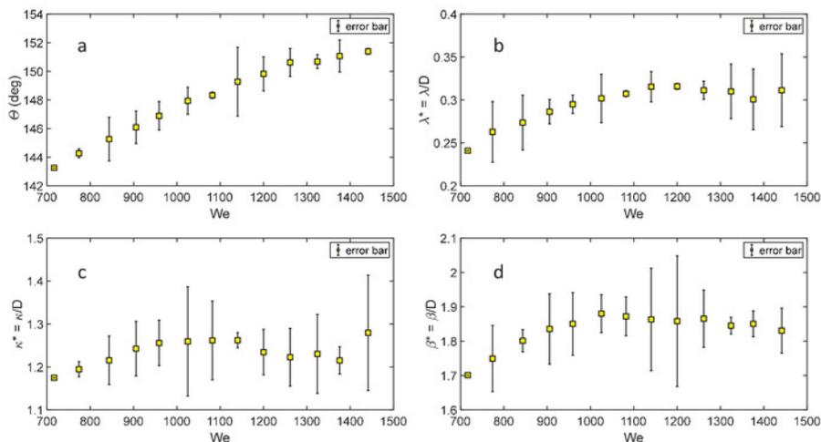
**Figure 4. Variation of cavity dimensions across Weber numbers.** Relation between  $We$  and the (a) separation angle  $\theta$ , (b) cavity depth  $\lambda$ , (c) splash crown height  $\kappa$ , and (d) cavity width  $\beta$ . Properties are non-dimensionalized in terms of sphere diameter,  $D$ . Error bars denote standard deviation for the average of five trials at each point. Figure is modified from Watson et al.<sup>1</sup>. [Please click here to view a larger version of this figure.](#)
